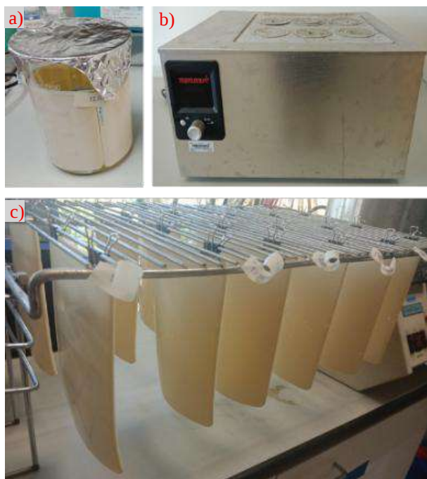
Figure 3: Leaching process: a) immersion in water or 1% SDS; b) incubation in a temperature-controlled water bath for 24 h; and c) drying at room temperature.
