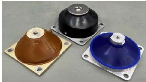
Figure 1. Tested Three Different Isolators
