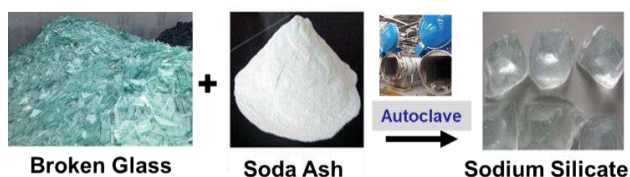
Figure 4. Wet process to produce sodium silicate from cullet.
