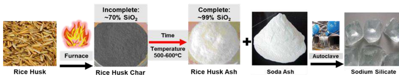
Figure 7. Steps to ash the bio-renewable rice husk to be used as a starting material to produce sodium silicate, then silica.
