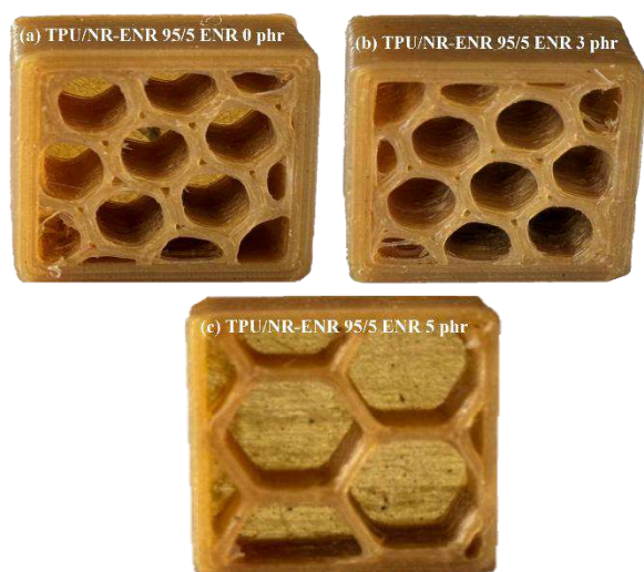
Figure 7 Printed TPU/NR-ENR (95/5 with 3 phr ENR) structures with varying parameters: (a) 15 mm/s, 3 walls; (b) 12 mm/s, 3 walls; (c) 7 mm/s, 2 walls, 7% infill.
