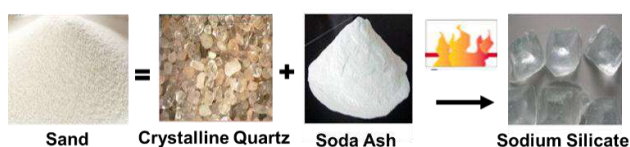
Figure 3. Dry furnace process to make sodium silicate from crystalline quartz (sand) by heating with soda ash.
