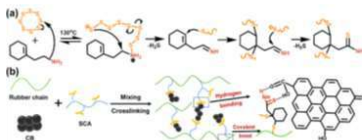
Figure 1. (a) Possible reaction pathways between 2-(1-cyclohexenyl) ethylamine (CA) and S 8 . (b) Proposed coupling mechanism between CB and rubber by SCA.
