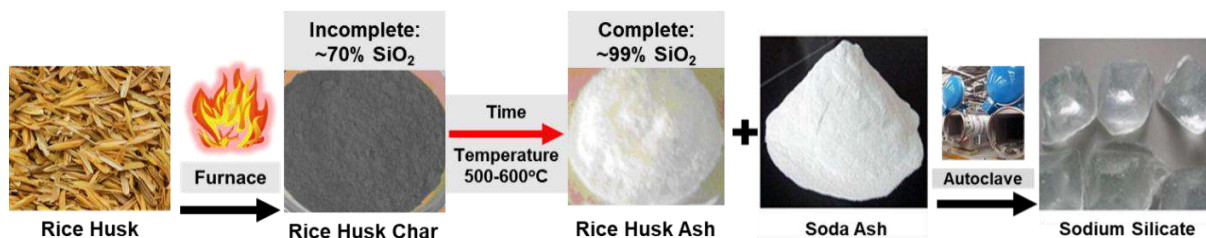
Figure 3. Furnace Process Ashes Renewable Rice Husk as Starting Material for Sodium Silicate.
