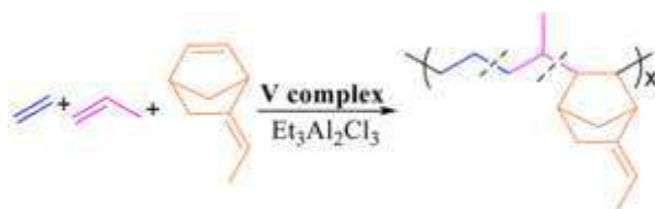
Figure 1. Terpolymerization of ethylene, propylene and ENB using V complex/ \text{Et}_3\text{Al}_2\text{Cl}_3 catalytic system
