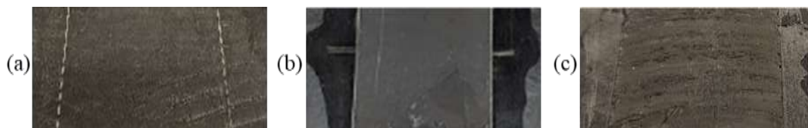
Figure 1. Failure types in peel tests: (a) adhesive, (b) transition with rubber film, (c) cohesive with rubber residue
