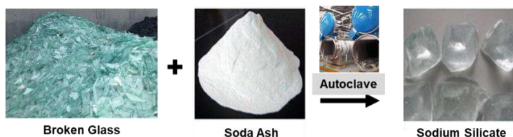
Figure 2. Wet (Autoclave) Process to make Sodium Silicate from Recycled Cullet (Broken Glass).
