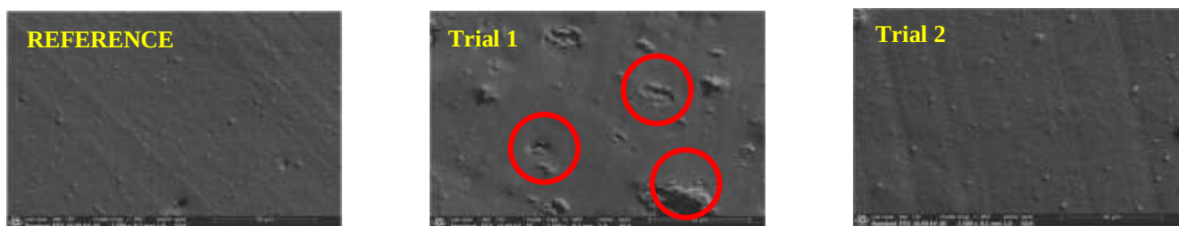
Figure 1: FESEM image showed that Trial 2 has comparable filler dispersion to the reference.
