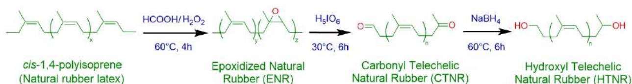
Figure 1. Synthesis of hydroxyl telechelic natural rubber (HTNR) from natural rubber
