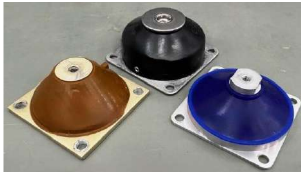
Figure 1. Tested Three Different Isolators
